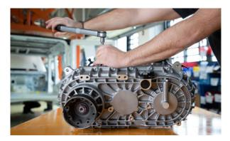
Despite the prevalence of SUVs on the road today, most are effectively two-wheel drive cars that switch into all-wheel drive when necessary. The Grenadier is a permanent fourwheel drive vehicle with high and low-range gearing. When it came to the transfer case, its requirements were very different from those of a road-going SUV.
