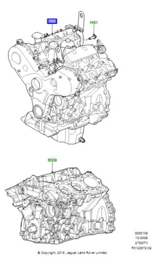
DISCOVERY 3 2005 - 2009 | SALLAAA139A512638 | |||| DISCOVERY 3 2005 - 2009 >> 2.7 Diesel V6 >> Powertrain >> 0301 Engine/Block, Heads & Manifolds >> 05 Service Engine And Short Block (Lion Diesel 2.7 V6 (140KW))((V)T09A999999)
