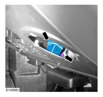
**11.** Carefully feed the new harness up to the ignition switch along the existing harnesses.
