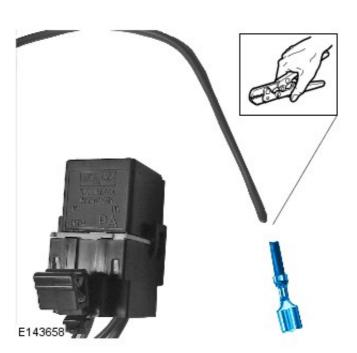
8. Cut the ground wire before the splice
