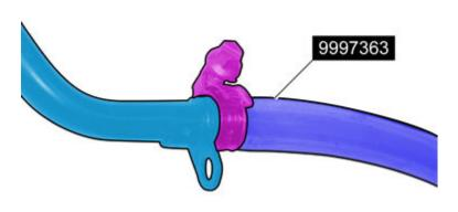
Install hose on the return line with a hose clamp.
