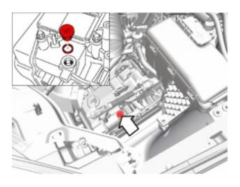
Remove the air cleaner (ACL) housing
