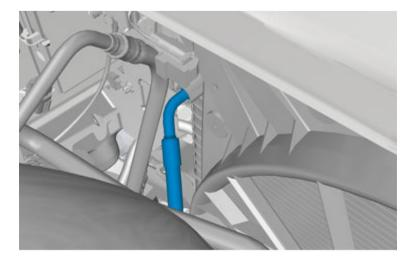
Remove the oil cooler's return line from the oil cooler.
