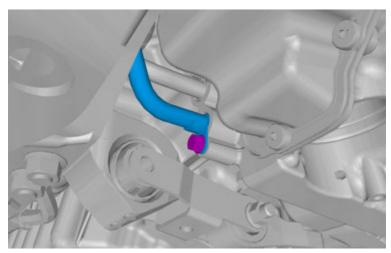
Remove the oil cooler's return line from the transmission.
