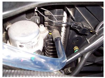
6 - Put the other end of the hose into premarked gallon jug. I put mine inside the bucket incase it spilled (which it did) and to make sure the jug wouldn't tip over.
