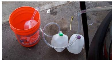
7 - Start the car and with the help of a friend pump out 2 quarts of oil at a time. I noticed that the XC90 pumped out slower than my 850 when I did that one.
