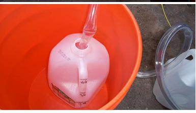
8 - After you have pumped out 2 quarts, turn the car off and refill 2 quarts. It doesn't matter so much that you pump out EXACTLY 2 quarts, you can be +/- on that, just so long as you end up with 12 out and 12 in. Be sure to factor in the oil that will be in the tube, not too much but be aware of it.
