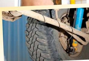
A displacement sensor was fitted alongside the shock to measure and record the exact movements of the shock during the off-road test track. The data was later replayed for each shock back on the dyn
