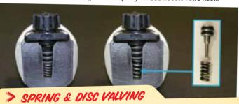
Spring and disc valving consists of a small, specially made coil spring that's fitted to the head of the piston. The spring holds a set pressure on a disc covering small ports in the piston head. This spring allows the disc to lift off the head of the piston, exposing the ports and allowing the flow of oil.
