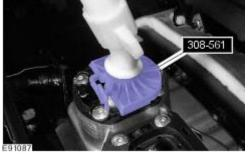
4 . Install a new differential lock pivot nut.
