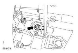
5 . Install the transfer case high/low range linkage. For additional information, refer to <u>Transfer Case High/Low Range Linkage</u>
