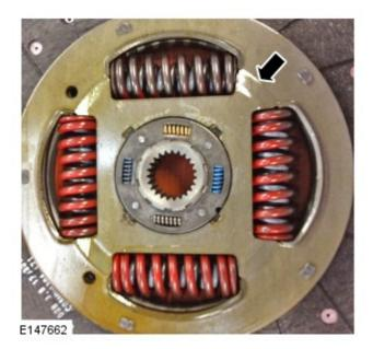
3. The new design clutch disc has a gloss finish and a bonded thrust washer.
