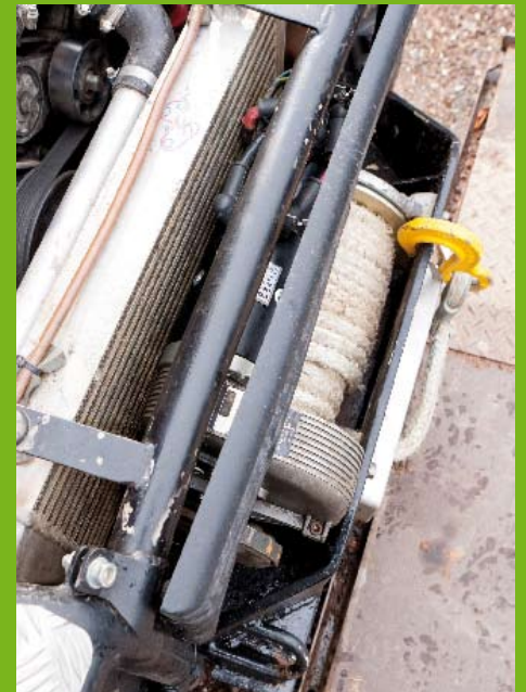
A Farr winch mount provides a neat home for the Warn 8274 on the front end, preventing what is a big, bulky bit of kit from imposing too much on the 90's famously good approach angle. The winch itself has an uprated mainshaft and brake from Giggiepin, as well as Allbright solenoids and a 9hp Bowmotor from Goodwinch. Needless to say, it runs Dyneema Bowrope for safety and ease of handling
