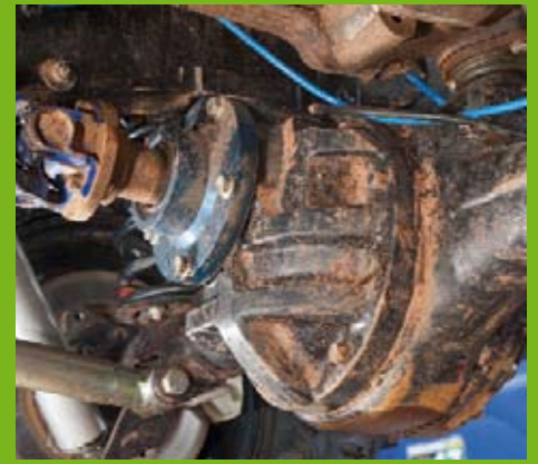
Both diffs are turned by heavy-duty, wide-angle 300Tdi propshafts from Gwyn Lewis
