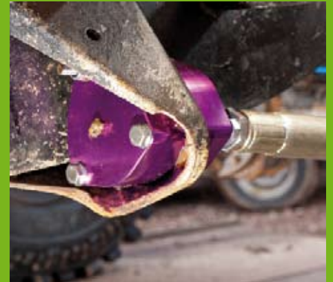
X-Eng says its adjustable rear radius arms allow more unrestricted articulation than any other trailing arm system on the market. You can fit them on any Defender, Mark 1 Disco or Range Rover Classic - but they're absolutely in their element on a hardcore challenge truck like James' trayback
