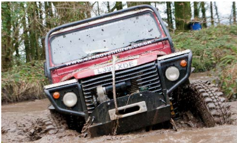
A Farr winch mount provides a neat home for the Warn 8274 on the front end, preventing what is a big, bulky bit of kit from imposing too much on the 90's famously good approach angle. The winch itself has an uprated mainshaft and brake from Giggiepin, as well as Allbright solenoids and a 9hp Bowmotor from Goodwinch. Needless to say, it runs Dyneema Bowrope for safety and ease of handling
