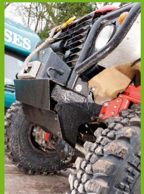
Thought we were joking about the approach angle? Turns out we weren't. Also on show here are front wing bars from North Off Road, which dial out one of the most vulnerable parts on any 90 that's going to get used hard
